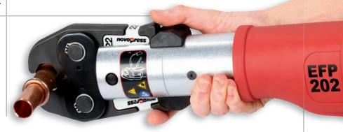
Before the beginning of the fitting deformation, the pressing cycle can be interrupted by releasing the start button. After the power build-up on the jaw, the piston will not return in its start position until the pressing cycle is completed - for high pressing safety. In case the pressing cycle needs to be interrupted, a release button can be actuated, for an immediately stop of the piston stroke.
