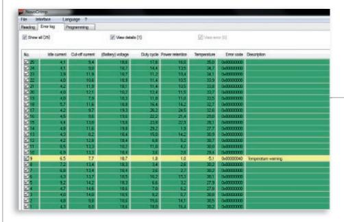
The NovoCrimp read tool can be used via USB interface to log all of the crimping operations performed and monitor correct performance.
